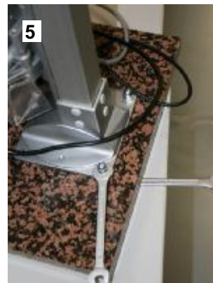
mounting the screws and nuts with both spanners
